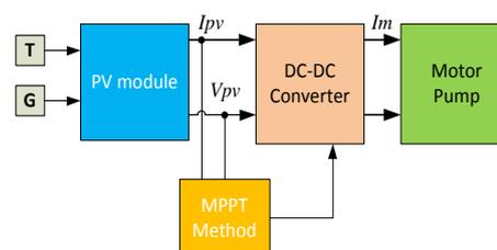
Fig 1. Diagram of MPPT in PV system
