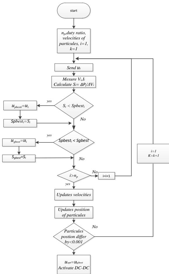
Fig 5. Flow chart of PSO algorithm.
