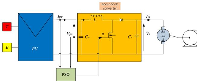
Fig 2. DC-DC Boost converter
